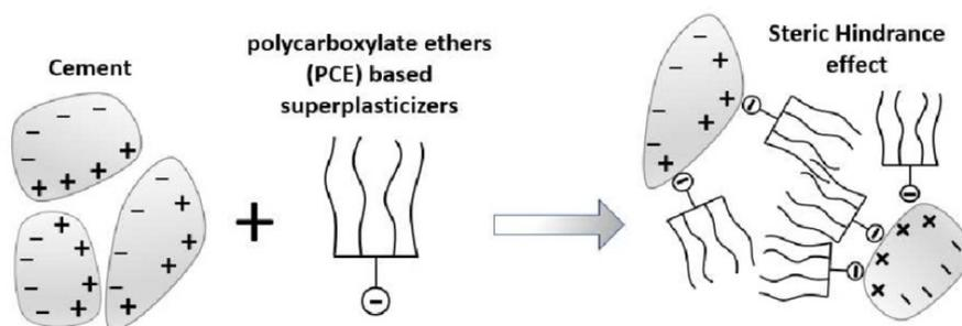
**Mid-Range Water Reducers** are classified as both Type A and Type F admixtures by ASTM C494. These are often low-power PCE's and are meant for 5-7" slumps (about 2" more than a normal-range water reducer would offer), and have a 5-18% water reduction. GCP's MIRA 62 is a common mid-range water reducer.
